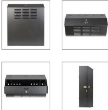
Wall-mount cabinet secures and organizes 5U of 19-inch rack equipment in network wiring closets and other locations with limited floor space. Houses equipment up to 20 inches deep, but extends less than 10 inches from wall.
